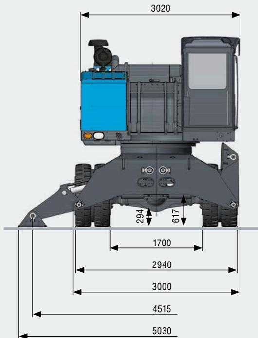
**TRANSPORT DIMENSIONS | TRANSPORTABMESSUNGEN | DIMENSIONS DE TRANSPORT [mm]**
