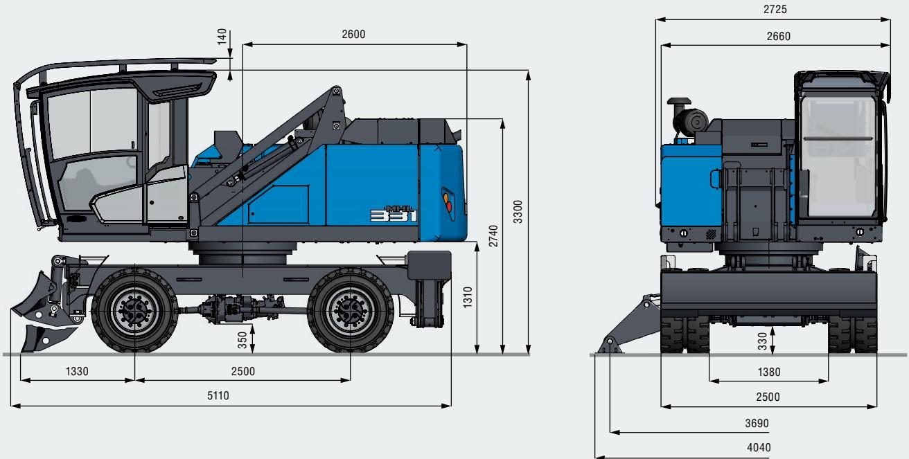
**TRANSPORT DIMENSIONS | TRANSPORTABMESSUNGEN | DIMENSIONS DE TRANSPORT [mm]****DIMENSIONES DE TRANSPORTES | DIMENSIONI DI TRASPORTO | DIMENSÕES DE TRANSPORTE [mm]**
