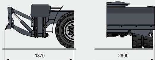
**2-point Stabilizers and support blade | 2-Punkt-Abstützung und Stützschild | 2 stabilisateurs et lame d'appui****Apoyo de 2 puntos y placa de apoyo | Sostegno a 2 punti e lama livellatrice di sostegno | Apoio em 2 pontos e placa de apoio**
